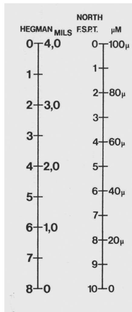
Figure 1 above shows the relationship between the various scales using the 1 to 100 $\mu$ m range as a guide. This diagram has been reproduced from the International Standard in order to show the simple conversion from the arbitrary scales to the micron scale.
